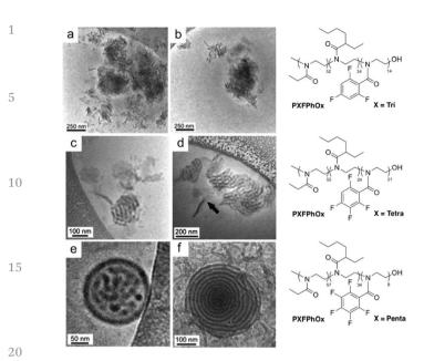
**Q16** Fig. 22 Cryo-TEM pictures of micellar aggregates formed by PEtOx-*b*-PEPOx-*b*-PXPhFOx triblock copolymers self-assembled in water. Adapted with permission from ref. 178. Copyright 2013 RSC.
