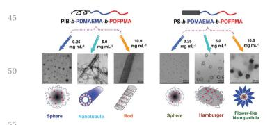
**Fig. 4** Schematic illustration and TEM images of numerous hierarchical assemblies formed from PIB-*b*-PDMAEMA-*b*-POFPMA and PS-*b*-PDMAEMA-*b*-POFPMA triblock terpolymers. Reproduced with permission from ref. 52. Copyright 2016 RSC.
