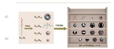
Fig. 9 (Left) Schematic representation of the PISA process and resulting morphologies obtained during the preparation of PDMAEMA-*b*-PBzMA micelles, worm-like and vesicles seeds. (Right) Compartmentalized nanostructures with a large variety of morphologies as a function of DP of PFHEMA (coined PTHFOMA in the text). Color code: D (red, PDMAEMA), B (grey, PBzMA), and H (black, PTHFOMA). Reproduced with permission from ref. 112. ACS 2017 Copyright.
