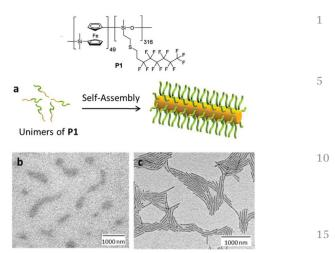
Fig. 26 Schematic representation of the self-assembly of PFS-b-PFMVS leading to cylindrical micelles. PFS = yellow, PFMVS functionalised with perfluoroalkane = light green (a). TEM micrographs of a drop-cast sample in TFT (60 mg mL<sup>-1</sup>) after 24 h (b) and 1 week (c). Reproduced 20 with permission from ref. 190. Copyright 2015 ACS.
