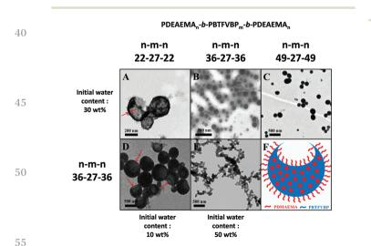
**Fig. 18** TEM images of morphologies formed from three different PDEAEMA-*b*-PBTFVBP-*b*-PDEAEMA triblock copolymers self-assembled in water when varying the initial water content. Adapted with permission from ref. 164. Copyright 2015 RSC.
