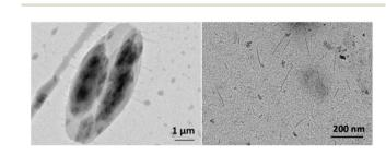
**Fig. 28** Desert rose-like morphologies synthesised through PISA (PVAc-*b*-PVDF BCs, left) and cylindrical rigid micelles (PVDF-*b*-PDMAEMA BCs, right) reported by Ladmiral *et al.*<sup>195,196</sup> Copyright 2017 RSC.
