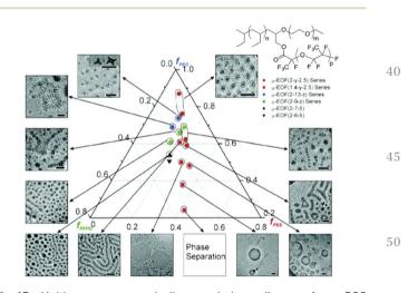
**Fig. 13** Multicompartment micelle morphology diagram for  $\mu$ -EOF miktoarm star terpolymers in dilute aqueous solution as a function of composition.  $f_{PEE}$ ,  $f_{PEO}$ , and  $f_{PFPO}$  are the volume fractions of the PEE, PEO, and PFPO blocks, respectively. They are designated  $\mu$ -EOF(x-y-z), where x, y, and z represent the E, O, and F block molar masses, respectively, in kD. Reproduced with permission from ref. 138. Copyright 2006 ACS.
