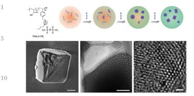
Fig. 29 (Top) BC structure and proposed self-assembly process of PAA-b-PIL in THF/H<sub>2</sub>O with the addition of water, resulting in the formation of cubosomes. (Bottom) SEM micrograph of the dried cubosomes after dialysis. (b) Cryo-TEM image of the [100] facet of a cuboid particle. (c) Enlarged surface image recorded in the central area of a cuboid particle from the [111] facet. Adapted with permission from ref. 204. Copyright Springer Nature 2016.
