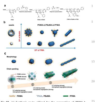
**Fig. 10** (a) Synthesis route utilized for the preparation of PDMA-*b*-PBZMA-*b*-PFDMA triblock copolymers. (b) Schematic representation of the obtained morphologies as a function of BZMA and PFDMA (FMA) degree of polymerisation (DPn). (c) Proposed mechanism for the formation of LC ordered morphologies with increasing PFDMA block length: PDMA<sub>33</sub>-*b*-PBZMA<sub>58</sub>-*b*-PFDMA<sub>16,30,62,120</sub> (from left to right). Adapted with permission from ref. 114. ACS 2017 Copyright.
