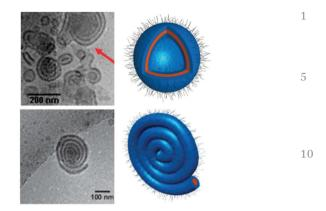
Fig. 21 Cryo-TEM pictures of micellar aggregates formed by the poly 15 (ODFOx<sub>23</sub>-b-EPOx<sub>28</sub>-b-EtOx<sub>49</sub>) triblock copolymer self-assembled in water. Adapted with permission from ref. 177. Copyright 2010 RSC.
