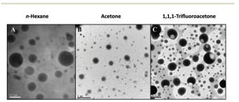
Fig. 17 TEM images of micelles formed by PBPFCBPMA-b-PIB-b-PBPFCBPMA triblock copolymers self-assembled in n-hexane (left), acetone (middle), and 1,1,1-trifluoroacetone (right). Adapted with permission from ref. 162. Copyright 2014 RSC.
