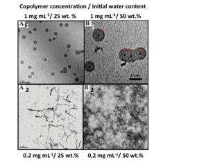
**Fig. 19** TEM images of the morphologies of PMBTFVB-*g*-PAA amphiphilic graft copolymers self-assembled in water when varying the initial water content and the concentration. Adapted with permission from ref. 166. Copyright 2015 RSC.
