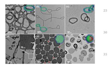
Fig. 27 TEM images of (a) toroids, (b) tadpoles and dumbbells, (c) interlocked toroids, (d and e) 2D nanosheets, and (f) laterally structured vesicles. FPOSS = red; PS = areen; PEO = blue. Reproduced with permission from ref. 191. Copyright 2015 ACS.
