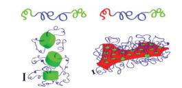
Fig. 14 Schematic representations showing the dependence of the network morphology on the end-blocks. 1,2-Polybutadiene, poly(ethylene oxide), and poly(perfluoropropylene oxide) are shown in red, blue, and green, respectively. The scale bars represent 5 nm. Adapted with permission from ref. 147. Copyright 2010 ACS.
