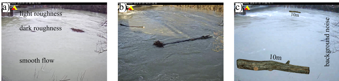
Figure 8. Different light conditions during (a) morning, (b) noon, and (c) late afternoon result in different frame roughnesses and different detection performances. (c) Wood position can highly affect the quality of detection. Pieces that are passing in front of the camera are detected much better than the pieces far from the camera.
