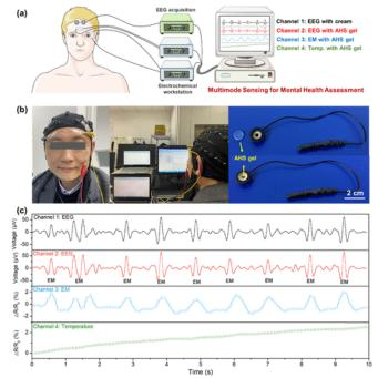
**Figure 5.** (a) Schematic illustration of multimode sensing for mental health assessment. (b) Fourchannel arrangement and the EEG probe using an as-prepared AHS hydrogel. (c) Time-dependent voltage and resistance change-based real-time monitoring for EEG, EM, and forehead temperature (the forehead of volunteer was precooled at 0 s).
