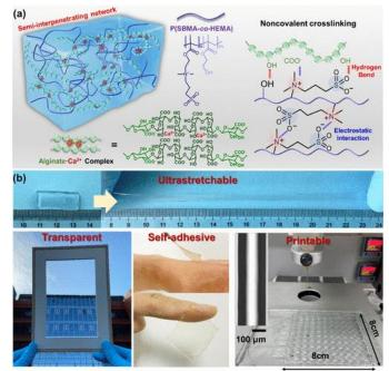
**Figure 1.** (a) Schematic illustration of the alginate/P(SBMA-*co*-HEMA) hydrogel (AHS) with a semiinterpenetrating network cross-linked by reversible noncovalent interactions. (b) Comprehensive fulfillment of its ultrastretchability, transparency, adhesion, and printability for dual force/temperature sensation.
