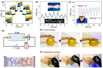
**Figure 4.** Time-dependent resistance change-based real-time monitoring for (a) finger bending at different angles, (b) pulse beat, and (c) vocal-cord vibration. (d) Schematic illustration of the hydrogel-based sensor with (e) force and (f) temperature dual-sensory capabilities for robotics when it approaches a (e) balloon and a (f) self-heating hot patch, respectively, based on the ionic conducting mechanism.
