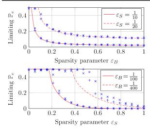
Figure 6. Limiting probability of error of spectral clustering of  $\mathcal{N}(\pm\mu,I_p)$  with equal class sizes on K: as a function of  $\varepsilon_B$  for fixed  $\ell=\|\mu\|^2=50$  (top), and  $\varepsilon_S$  for fixed  $\ell=50$  (bottom). Simulations (single realization) in markers for  $p=n=4\,000$  (×) and  $p=n=8\,000$  (+). Very good fit between theory and practice for not too small  $\varepsilon_S,\varepsilon_B$ .
