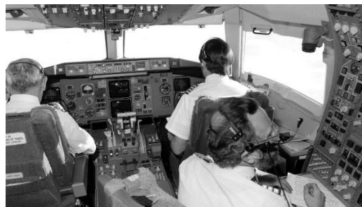
Figure 1. Cockpit of an airbus A300 with pilot flying, pilot monitoring and flight engineer
