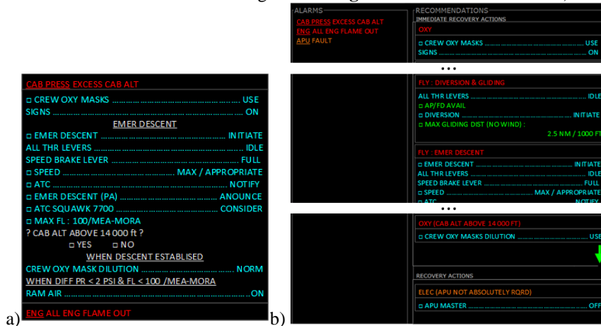
Fig. 3. FWS user interface prototypes a) A350-FWS user interface prototype b) REC-FWS user interface prototype
