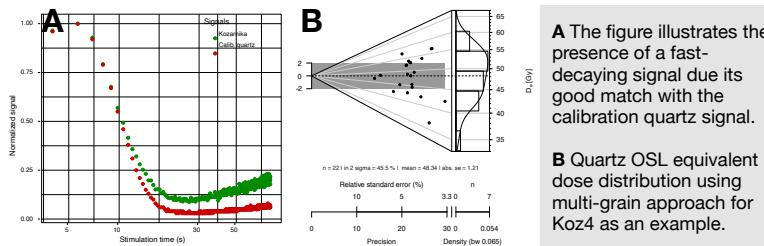
A The figure illustrates the presence of a fast-decaying signal due its good match with the calibration quartz signal.
