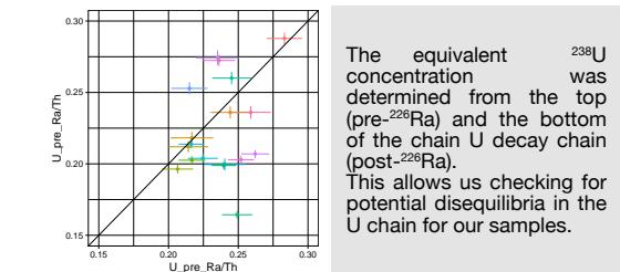
The equivalent <sup>238</sup>U concentration was determined from the top (pre-<sup>226</sup>Ra) and the bottom of the chain U decay chain (post-<sup>226</sup>Ra). This allows us checking for potential disequilibria in the U chain for our samples.
