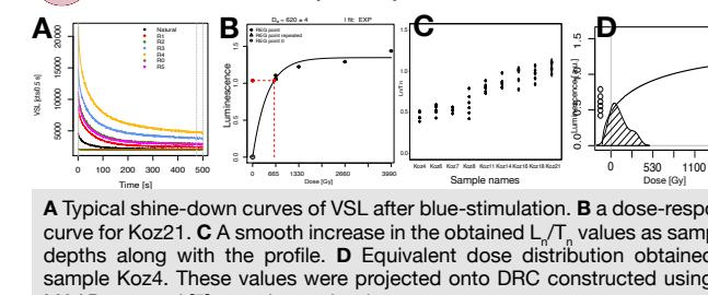
A Typical shine-down curves of VSL after blue-stimulation. B A dose-response curve for Koz21. C A smooth increase in the obtained  $L_n/T_n$  values as samples' depths along with the profile. D Equivalent dose distribution obtained for sample Koz4. These values were projected onto DRC constructed using the MAAD protocol [5] to estimate the dose response.
