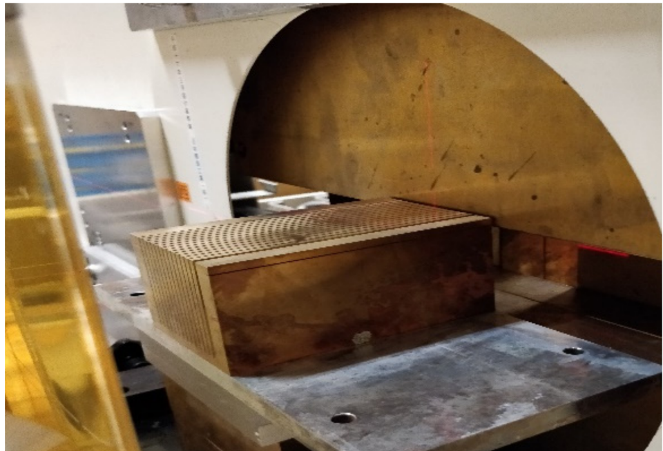
Figure 1. Photograph of the multislit brass collimator placed at the jaws exit of the beamline at biology room of HIMAC.
