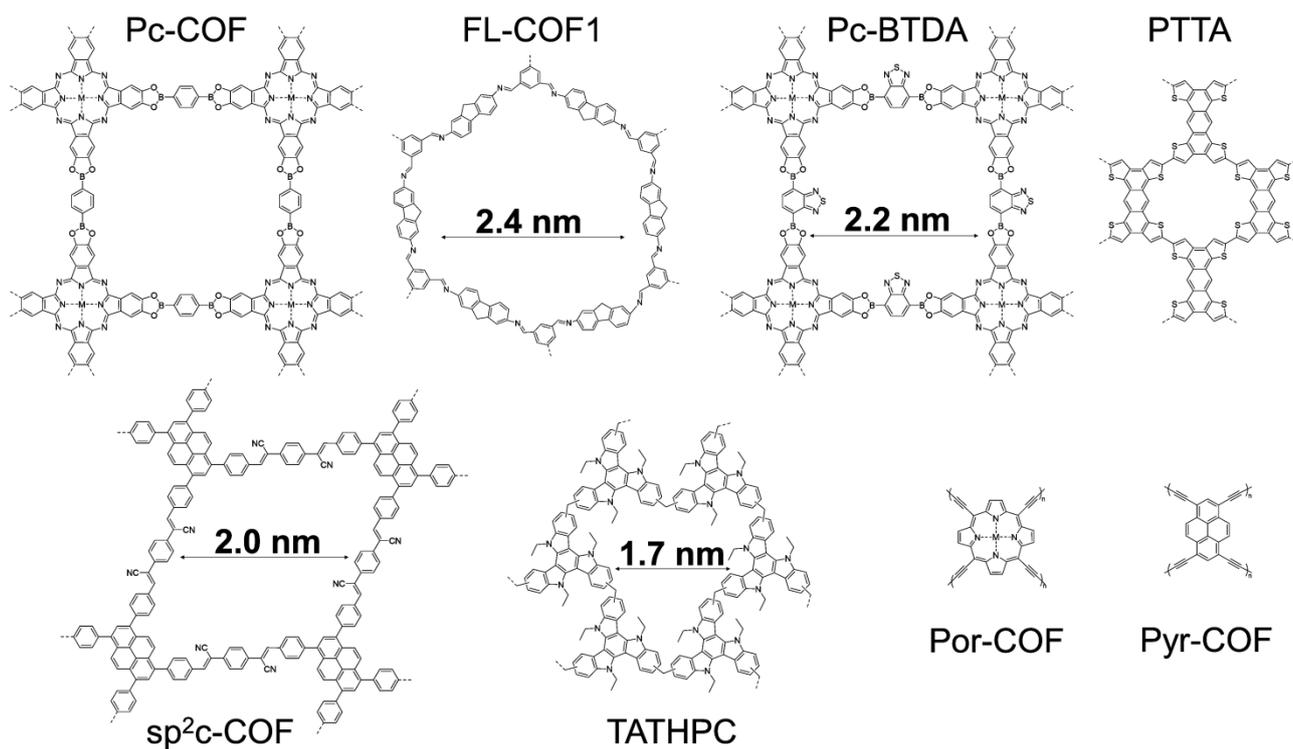
Figure 4: Chemical structure of COFs and HPC.
