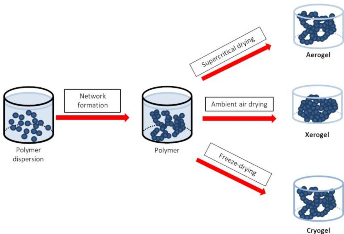
Figure 2: Schematic routes to fabricate polymer gel network and dried gels, case of PEDOT:PSS. The polymer chains are represented by the dark blue beads while the solvent (water) is in light blue.
