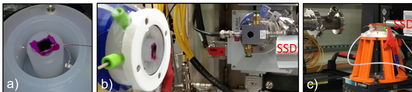
Figure 1. Electrochemical cell used for the x-ray in situ studies. (a) Dry cell, without Mylar foil, with sample mounted contacted by gold wire. (b) Cell filled with electrolyte, mounted on diffractometer; SSD shown removed from the sample. (c) Cell mounted on B16 with XRF detected at grazing exit angle of about 5^\circ .
