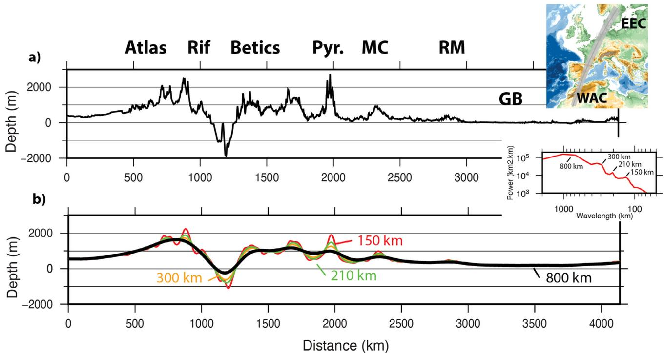
**Fig. 4.** Topography of Western Europe and filtered wavelengths of topography. A low-pass filter was applied on the total topographic (a) so the residual topography (b) contains only wavelengths larger than 150, 210, 300 and 800 km. Inset shows the dominant wavelengths obtained by the power spectral density analysis.
