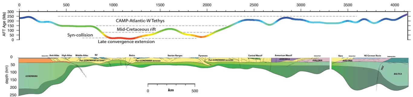
**Fig. 15.** Distribution of apatite fission-track (AFT) age after data gridding extracted along profile 1 (see location in Fig. 12), same color coded as Figure 12. Below is the structural section of reference presented in Figures 10 and 11.
