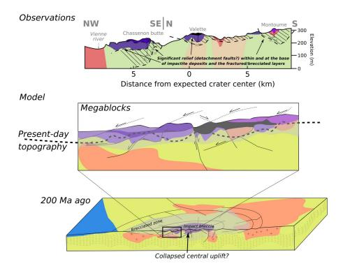
Figure 7. (Top) Geological cross section of Figure 1, with constraints from this study, (middle) interpreted schematic 2D model of the Chassenon area (showing megablocks and tilting), and (bottom) its eventual position within the whole Rochechouart impact structure about 200 Ma ago.
