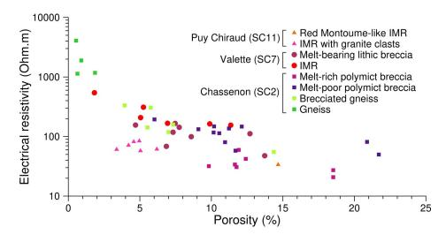
Figure 4. Electrical resistivity versus porosity of core samples from SC2 (Chassenon), SC7 (Valette), and SC11 (Puy Chiraud) drilling sites.
