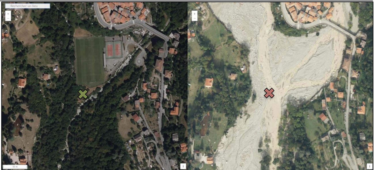
Figure 2: Aerial photography of Saint-Martin-Vésubie, before the 2020 flood (left picture), and a few days after the event (right). The marker at the center of the picture is the location of a Météo-France SWS, that has been destroyed by floods. Source: alex.ign.fr (IGN)
