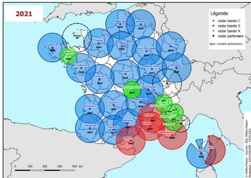
**Figure 3:** Météo-France weather radar network in February 2021. There are 20 C-band radars, 5 S-band radars, 6 X-band radars (+2 at Paris CDG and Nice airports). The network is extended with 3 partner radars, one of them particularly interesting in our area of interest (X-band radar of Mont Vial, operated by the company NOVIMET), which allow a better coverage of the Mercantour area. Source: Météo-France
