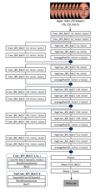
Figure 3. The framework of spatio-temporal networks for pulse rate estimation directly from facial videos recording.
