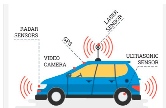
Figure 5. data fusion and machine learning are hugely important for detecting and identifying both static and dynamic targets. Excerpted from reference [45].
