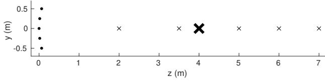
Figure 6: Geometry of the array ensuring unbiased range estimation of the source at  $z = 4\text{m}$ . Microphones in the plane  $x = 0$  indicated by disks, sources positions used in figure 7 by crosses.
