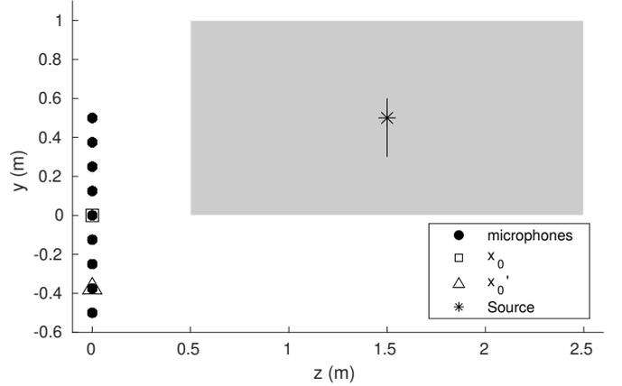
Figure 1: Geometry of the problem. Region of interest for Figure 2 indicated by the grey rectangle. The line on which the source is search in Figure 3 is indicated.
