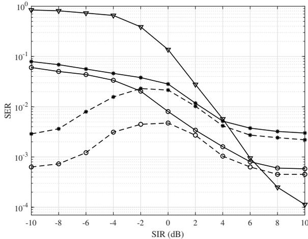
Fig. 7: SER as a function of the SIR for the *classical detector* [▽], the *DFNN-based* [∗], and the *CNN-based* [○]. The SNR for the selected user is set to  $-6$  dB. Two different cases are considered: plots in solid line [—] *networks trained for  $\lambda = 0.25$* , plots in dashed line [--] *networks trained for each SIR value*.
