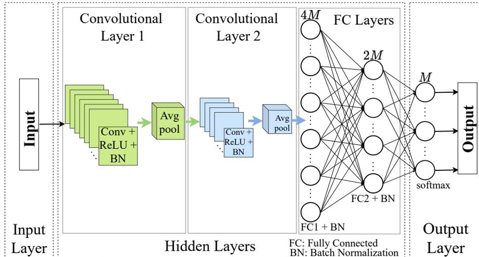
Fig. 4: Convolutional Neural Network architecture.
