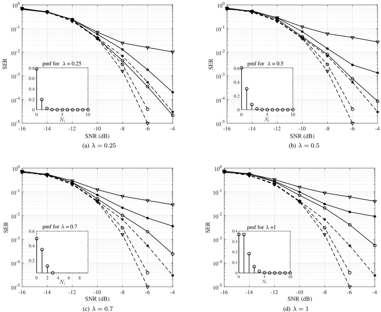
Fig. 6: Symbol error rate as a function of the SNR for different detection approaches: *classical decoder* [ $\nabla$ ], *DFNN-based* [ $*$ ], and *CNN-based* [ $\circ$ ]. For all figures, two scenarios are considered: *no interference* (plots in dashed line [- -]) and *when interference can happen* (plots in solid line [—]). The plot inside show the probability mass function (pmf) related to the number of interfering users.
