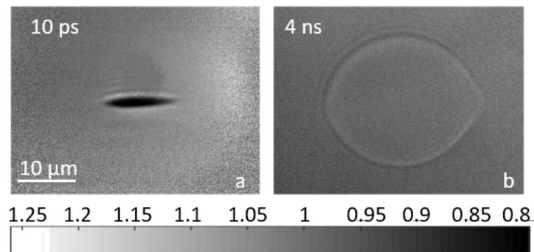
**Fig. 1** Experimentally obtained transmission images in air following excitation by a single 5- $\mu\text{J}$  femtosecond pulse. Two delays after the arrival of the pulse are displayed: 10 ps (a) and 4 ns (b).
