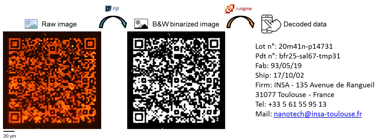
Figure S.2 Image processing and reading sequence of a QR code based on 3D assembly of HNPs.
