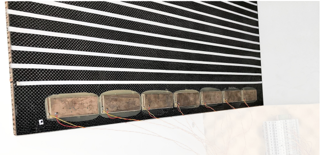
FIG. 7. Picture of the actuators' array for 8th-order guided resonance actuation.
