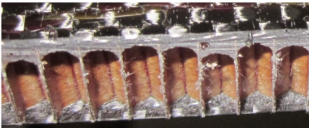
Figure 5: Picture of a section of the sandwich panel, the width is the  $W$ -direction.
