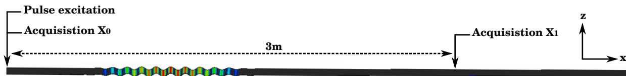
Figure 2: Illustration of the numerical procedure for measuring the group velocities in the beam. Simulations are conducted using the FEA package Abaqus CAE V6.13 with Abaqus/Explicit solver. Linear C3D8 elements are used and a minimum mesh density of 15 elements per wavelength is applied, leading to a 120000 elements model at 13.2 kHz. Note that the choice of a beam is motivated by the elevated computational times associated with 2D transient simulations.
