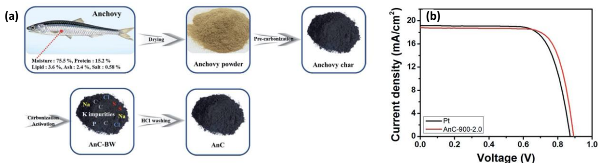
Figure 7. (a) Preparation of anchovy-derived nitrogen and sulfur co-doped carbon materials, and (b) the J-V curves of the DSCs with Pt (black curve) and AnC (N,S co-doped-AC) counter-electrodes (red curve). Figure reproduced from Kim et al. 42 with permission from Royal Society of Chemistry.
