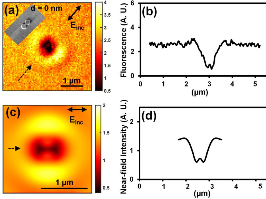
Figure 5. Experimental fluorescence image (a) and cross-section (b) measured on a structure with touching nanodisks ( $d = 0$  nm); FDTD simulation (c) and cross-section (d) of the electromagnetic field intensity on the structure. The inset in (a) is a SEM image of the dimer.
