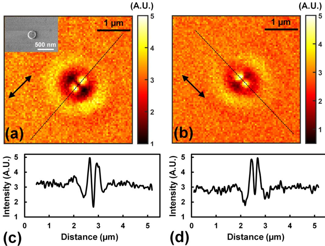
Fig.2 Near-field fluorescence maps (a,b) and cross-sections (c,d) measured when a nanocrystal is scanning an isolated 240 nm-large gold nanodisk. The excitation was performed at  $\lambda_{\text{EXC}} = 975$  nm and the luminescence was detected in the 520-550 nm range. The incident polarization of the laser beam is indicated by the arrow. The inset is an SEM picture of the nanodisk.
