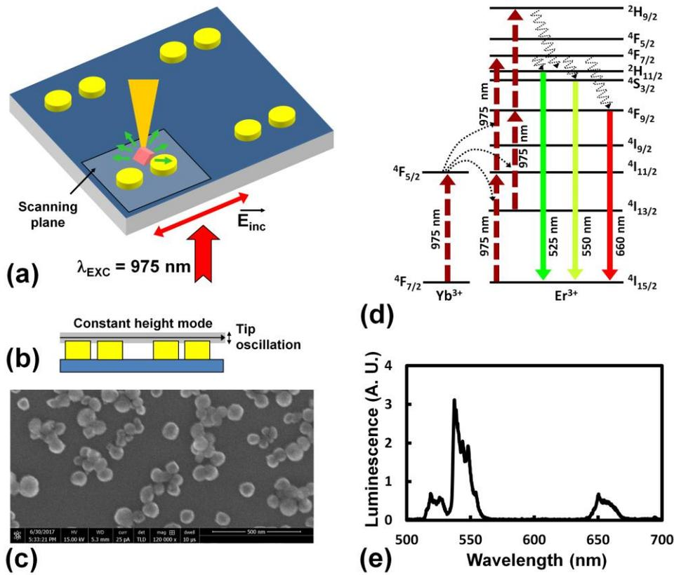
Fig.1. Sketch of the illumination configuration (a) and the scanning mode (b), SEM image of a 100-150 nm large fluorescent  $\text{NaYF}_4:\text{Er}^{3+}/\text{Yb}^{3+}$  nanocrystals (c), energy band diagram (d) and luminescence spectrum of the nanocrystals. The excitation was performed at  $\lambda_{\text{EXC}} = 975$  nm.
