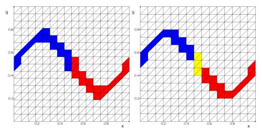
Figure 14: Test case with a crack, meshes used for  $\phi$ -FEM. Left: a mesh resolving the crack tip; the cells in  $\mathcal{T}_h^{\Gamma_{int}}$  in blue; the cells in  $\mathcal{T}_h^{\Gamma_f}$  in red. Right: a mesh not resolving the crack tip; in addition to blue and red cells, there are yellow cells not belonging to  $\mathcal{T}_h^{\Gamma_{int}}$  or  $\mathcal{T}_h^{\Gamma_f}$ .
