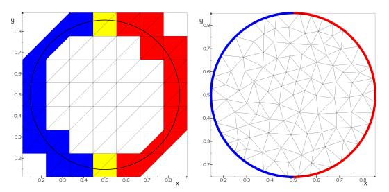
Figure 8: Test case with mixed boundary conditions, meshes not resolving the Dirichlet/Neumann junction. Left: active meshes for  $\phi$ -FEM, red for  $\mathcal{T}_h^{\Gamma_D}$ , blue for  $\mathcal{T}_h^{\Gamma_N}$ , yellow for  $\mathcal{T}_h^{\Gamma}$  otherwise unmarked. Right: a mesh for standard FEM, red boundary facets on  $\Gamma_D$ , blue boundary facets on  $\Gamma_D$ , note that some boundary facets contain both Dirichlet and Neumann parts.
