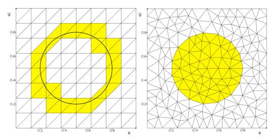
Figure 11: Linear elasticity with multiple materials. Left: a mesh used for  $\phi$ -FEM ( $\Omega_h^{\Gamma}$  painted in yellow); Right: a mesh matching the interface for standard FEM (yellow and white represent the two materials).
