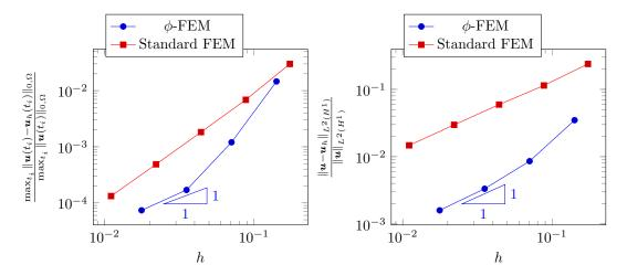
Figure 16: Test case for the heat equation;  $\Delta t = h$ . Left:  $L^{\infty}(0,T;L^{2}(\Omega))$  relative errors. Right:  $L^{2}(0,T;H^{1}(\Omega))$  relative errors.
