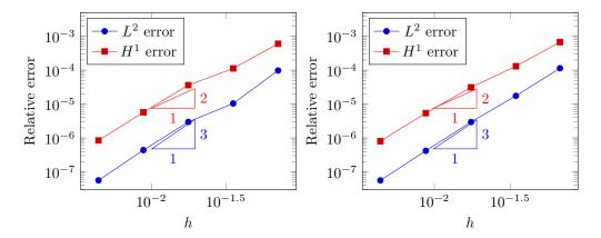
Figure 15: Test case with a crack,  $H^1$  and  $L^2$  relative errors. Left: on meshes resolving the crack tip. Right: on meshes not resolving the crack tip.
