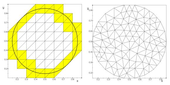
Figure 2: Circular domain given by (20). Left: active meshes for  $\phi$ -FEM (with cells from  $\mathcal{T}_h^{\Gamma}$  in yellow). Right: a fitted mesh for the standard FEM.
