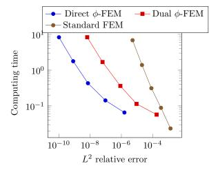
Figure 4: Test case with pure Dirichlet conditions. Computing time (in seconds) vs. the  $L^2$  relative errors.
