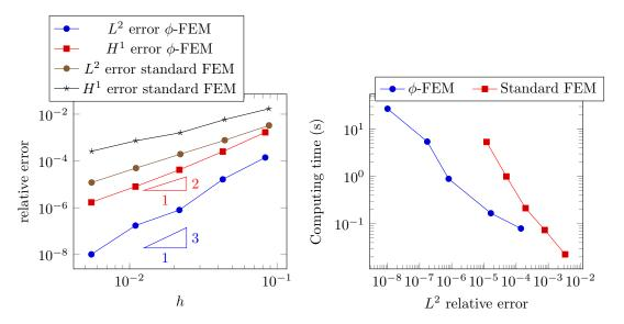
Figure 9: Test case with mixed boundary conditions, results on meshes as on Fig. 8. Left:  $L^2$  and  $H^1$  relative errors under the mesh refinement. Right: computing time vs. the  $L^2$  relative error.
