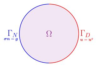
Figure 5: Test case with mixed boundary conditions: the geometry of Dirichlet and Neumann boundary parts.
