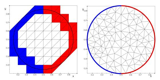
Figure 6: Test case with mixed boundary conditions, meshes resolving the Dirichlet/Neumann junction. Left: active meshes for  $\phi$ -FEM, red for  $\mathcal{T}_h^{\Gamma_D}$ , blue for  $\mathcal{T}_h^{\Gamma_N}$ . Right: a mesh for standard FEM, red boundary facets on  $\Gamma_D$ , blue boundary facets on  $\Gamma_N$ .
