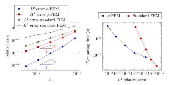
Figure 7: Test case with mixed boundary conditions, results on meshes as on Fig. 6. Left:  $L^2$  and  $H^1$  relative errors under the mesh refinement. Right: computing time vs. the  $L^2$  relative error.
