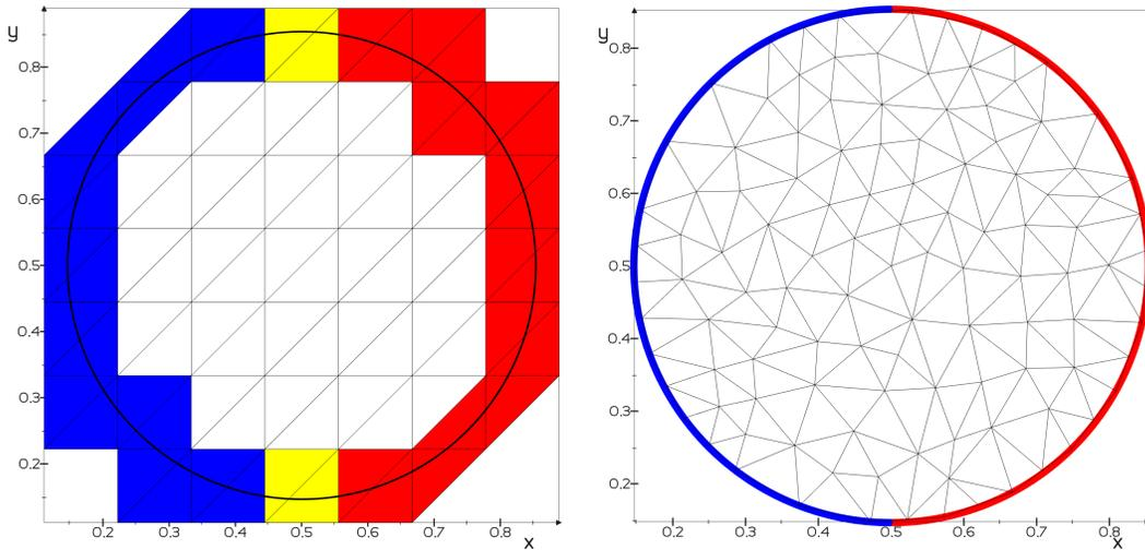
Figure 8: Test case with mixed boundary conditions, meshes not resolving the Dirichlet/Neumann junction. Left: active meshes for  $\phi$ -FEM, red for  $\mathcal{T}_h^{\Gamma_D}$ , blue for  $\mathcal{T}_h^{\Gamma_N}$ , yellow for  $\mathcal{T}_h^{\Gamma}$  otherwise unmarked. Right: a mesh for standard FEM, red boundary facets on  $\Gamma_D$ , blue boundary facets on  $\Gamma_N$ , note that some boundary facets contain both Dirichlet and Neumann parts.
