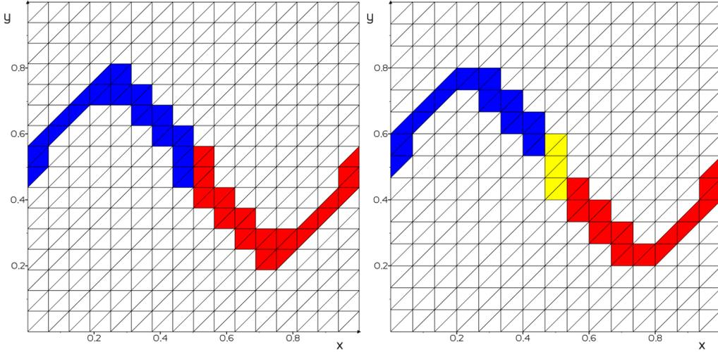
Figure 14: Test case with a crack, meshes used for  $\phi$ -FEM. Left: a mesh resolving the crack tip; the cells in  $\mathcal{T}_h^{\Gamma_{int}}$  in blue; the cells in  $\mathcal{T}_h^{\Gamma_f}$  in red. Right: a mesh not resolving the crack tip; in addition to blue and red cells, there are yellow cells not belonging to  $\mathcal{T}_h^{\Gamma_{int}}$  or  $\mathcal{T}_h^{\Gamma_f}$ .
