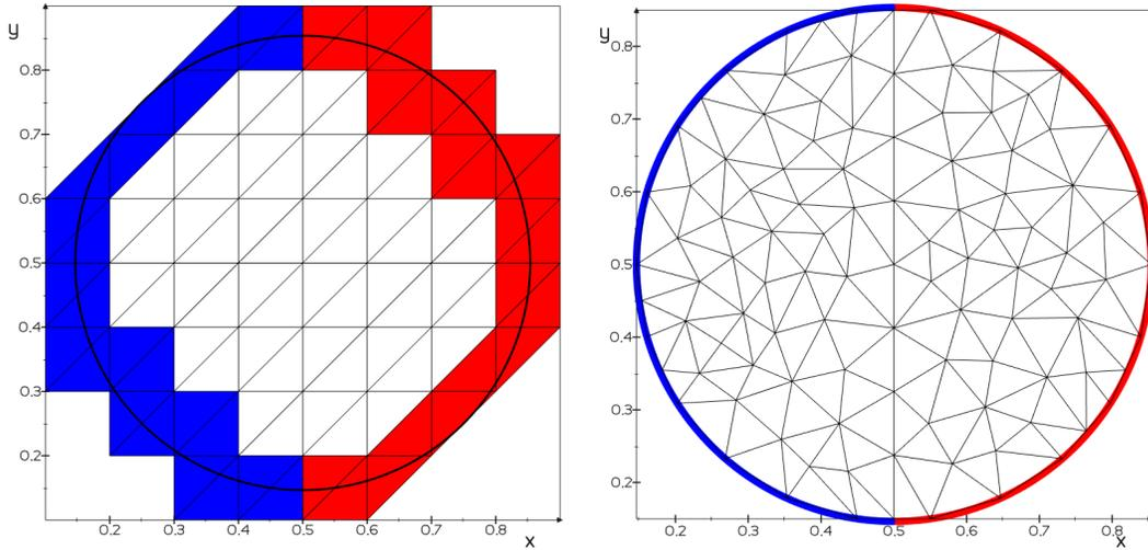
Figure 6: Test case with mixed boundary conditions, meshes resolving the Dirichlet/Neumann junction. Left: active meshes for  $\phi$ -FEM, red for  $\mathcal{T}_h^{\Gamma_D}$ , blue for  $\mathcal{T}_h^{\Gamma_N}$ . Right: a mesh for standard FEM, red boundary facets on  $\Gamma_D$ , blue boundary facets on  $\Gamma_N$ .
