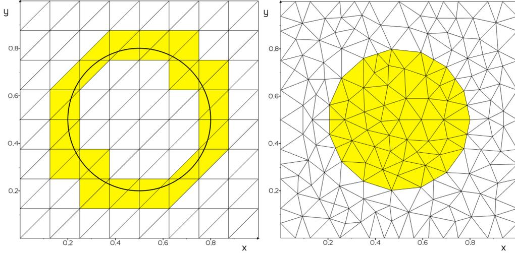
Figure 11: Linear elasticity with multiple materials. Left: a mesh used for  $\phi$ -FEM ( $\Omega_h^\Gamma$  painted in yellow); Right: a mesh matching the interface for standard FEM (yellow and white represent the two materials).
