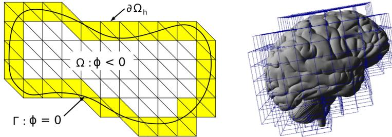
Figure 1: Left: Meshes and notations for a 2D domain  $\Omega = \{\phi < 0\}$ ; the computational mesh  $\mathcal{T}_h$  is obtained from a structured background mesh and is represented by both white and yellow triangles forming the domain  $\Omega_h$ ; the yellow triangles constitute the submesh  $\mathcal{T}_h^\Gamma$  occupying the domain  $\Omega_h^\Gamma$ . Right: a more involved example of an active mesh in 3D that can be used in  $\phi$ -FEM; a hexahedral mesh covering a brain geometry.
