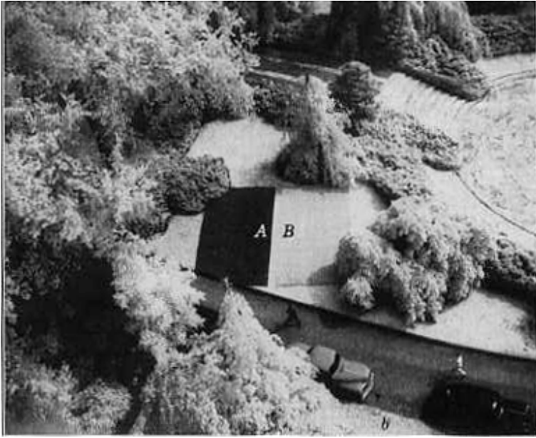
Fig. 9: Camouflage detection: (a) photograph of painted panel against a background of grass on panchromatic film, and (b) by infrared (from Clark 1946).
