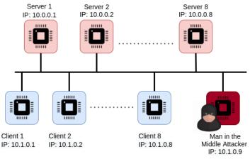
Fig. 2. Configured Network - Different SOME/IP clients and servers exchanging SOME/IP services over Automotive Ethernet Bus. Besides, a Client ECU is being compromised by an MITM Attacker.
