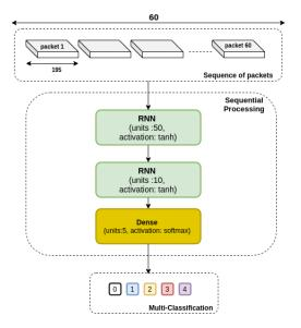
Fig. 5. RNN based IDS architecture
