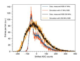
Figure 2: Measured and simulated pedestal shapes of two specific pixels with different NSB levels as a function of the charge (centered around 0).
