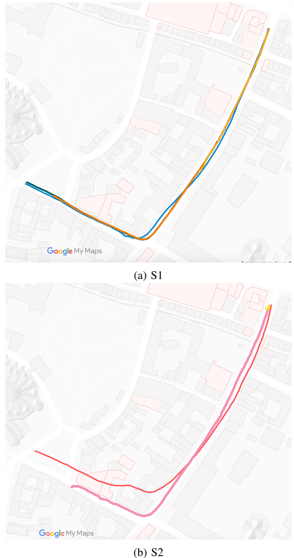
Fig. 5: Direct 3D model-based tracking with PGMoT and PoT with the camera aboard a vehicle: Estimated trajectories for (a) the first sequence S1 (GPS: blue; Camera poses output of the photogrammetry process: dark green; PGMoT: orange; PoT: yellow) and (b) the second sequence S2 (GPS: red; PGMoT: pink; PoT: yellow). Trajectories are plotted after conversion to latitude and longitude coordinates exported as kml files to Google My Maps (base map monochrome).
