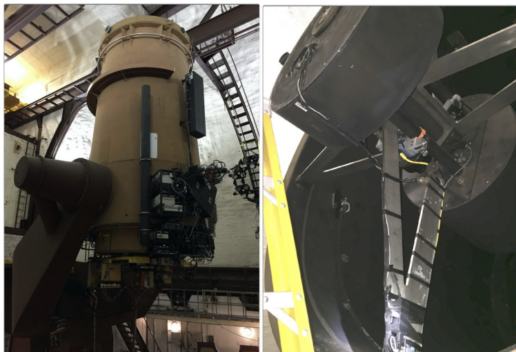
Figure 1. (LEFT) The University of Hawaii 2.2-meter telescope (LEFT) shown with the Robo-AO system mounted to the North bent-Cassegrain port. The Robo-AO Rayleigh laser is the long black rectangular box seen midway up the side of the telescope tube. (RIGHT) The top-end of the telescope showing its two secondary mirrors. The secondary currently “in the beam” is the f/10 fixed secondary. The secondary out of the beam (pointed away from the telescope tube) is the no longer used Coude secondary. The UH88 ASM will replace this Coude secondary. The top-end can rotate ( \sim 30 min) to place either secondary in the beam.
