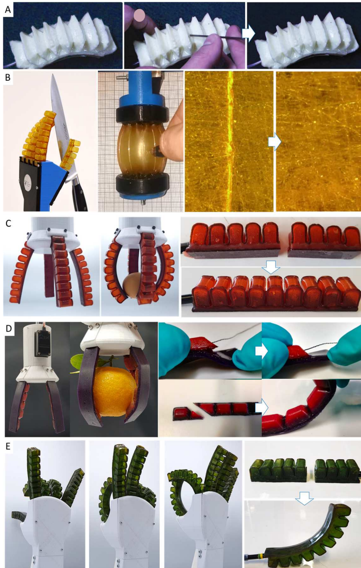
Figure 6: A) Soft bending actuator, constructed out of a silicone/Kevlar composite, that is resistant to small punctures due to self-sealing based on the self-adhesion of silicone (219). B) A soft pneumatic hand (125) and pleated pneumatic artificial muscle (127) that are given an intrinsic healing capacity by constructing them out of Diels-Alder elastomers. Cuts and perforations are healed by subjecting the parts to 80 °C for 40 minutes. C and D) Different types of soft grippers, pneumatically actuated (126) or tendon driven (123), that are constructed out of multiple Diels-Alder polymers. Large cuts, including ones that damage more than one material section, as well as damage due to delamination at multi-material interfaces, can be healed by heating the parts to 90 °C for 30 to 40 minutes. The performance of these robotic components is not influenced by a damage-heal cycle. E) A soft pneumatic robotic hand manufactured out of a Diels-Alder based network that can autonomously heal at room temperature (121). Large damages, like cutting fingers in halve are healed without decreasing the systems performance.
