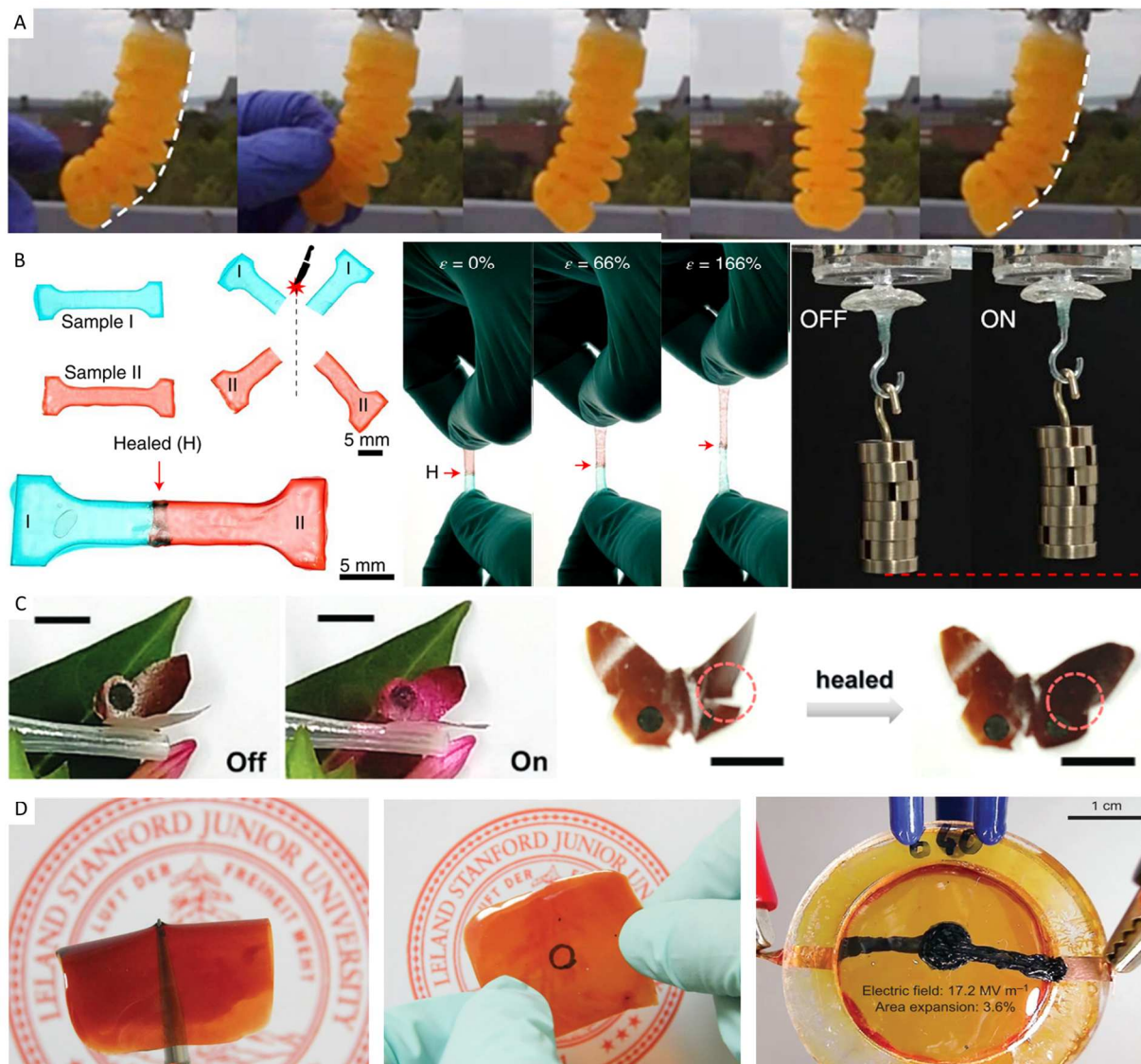
Figure 8: A) A soft pneumatic bending actuator manufactured out PDMS using stereolithography (228). During the manufacturing process, uncured thiolene resin is encapsulated. The actuator is hydraulically actuated by pressurizing the unreacted resin. When the membrane is perforated, the thiolene resin escapes. In contact with oxygen and in the presence of visible light the thiolene resin polymerizes and acts as a healing agent, sealing the damage. B) Squid-inspired synthetic proteins were used to generate supramolecular networks that are physically crosslinked by crystalline phases with extensive hydrogen bonds (211). The networks have high mechanical strength and can heal large damages at 50 °C in the order seconds. These elastomers were used to develop the first protein-based self-healing actuator. C) Y. Wang et al. developed multi-stimuli responsive actuators with healing capacities relying on both hydrogen bonds and ferric oxide–catechol (metal-ligand) complexes (210). The combination of these physical crosslinks allows healing at room temperature as illustrated in a butterfly prototype that is actuated by local heating through irradiation of near-infrared light and due to mismatch in the coefficient of thermal expansion between different layers in the material. D) A self-healing dielectric actuator in which the dielectric layer is a Fe(III)-pdca (metal-ligand) based self-healing elastomer (189). Defects in the dielectric medium are healed before they propagate can prevent dielectric breakdown.
