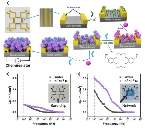
**Fig. 6.** 0D electrical sensor-based of networks of Au NPs for K<sup>+</sup> sensing (a) Schematic layerby-layer fabrication of CRs based on covalently assembled Au NPs-DTDB-18C6 networks, Capacitance response of (b) bare and (c) Au NPs-DTDB-18C6 network-coated IDEs in Milli Q water (black curves) and K<sup>+</sup>  $10^{-3}$  M (violet curves). Inset: Respective pictures of the bare and network-coated glass chips. Adapted from ref.<sup>98</sup> with permission from Wiley-VHC.
