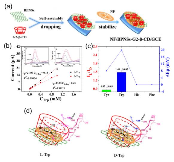
**Fig. 12.** 2D BP-based electrochemical sensing for enantiomeric discrimination. (a) Fabrication of the modified glassy carbon electrodes (GCE) with BP nanosheets functionalized with G2-β-CD and stabilized with Nafion (NF). (b) Sensor electrochemical response to D- and L-tryptophan (Trp). (c) Sensor current and potential ratio for the enantiomeric discrimination of
