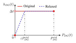
Fig. 4. Diesel generator operation hours models.
