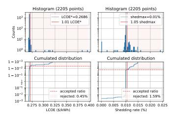
Fig. 5. Distribution of the multi-start optimization results for one test case  $(\varepsilon=0.1,\,SR^{max}=0.01\,\%)$ . Distribution of the objective on the left and of the constraint on the right. Distributions are shown as log-scaled histograms on top and as cumulated distributions on the bottom, with a "logit" scale to highlight frequencies close to 0 and 1. Vertical red lines are tolerance thresholds for counting results as acceptable.
