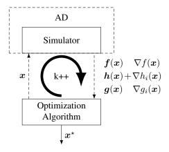
Fig. 2. Relation between optimizer and simulator.
