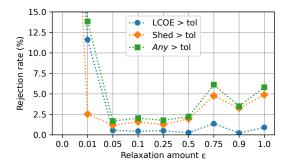
Fig. 6. Effect of the amount of relaxation  $\varepsilon$  on the rejection rate of optimization results (case  $SR^{max}=0.01\,\%$ ). Values for  $\varepsilon=0$  are out of bounds because all points are rejected.
