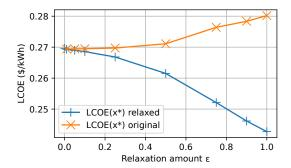
Fig. 7. Effect of the relaxation on biasing the optimal sizing (case  $SR^{max}=0.01\,\%$ ). The best sizing (among all multistarts) for a given amount of relaxation  $\varepsilon$  is evaluated in the unrelaxed simulator. For  $\varepsilon\geq 0.25$ , the relaxed optimal sizing is too far from the actual unrelaxed optimum, so that it yields a too large unrelaxed cost.
