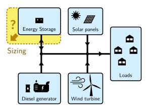
Fig. 1. Islanded microgrid architecture considered in this work. The microgrid sizing problem is about finding the optimal ratings of *all* its components.
