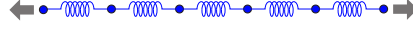
Figure 1: The simplest (not reinforced) mass-spring chain. Particles are connected in series by breakable springs and the whole system is loaded in tension.
