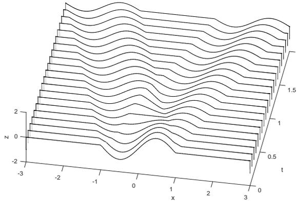
**Fig. 1** Free evolution of the linear wave equation.
