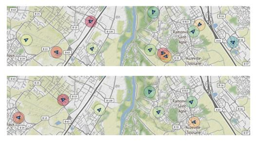
Fig. 3 Conflict-free trajectories (bottom) generated to minimize bubbles' intersections (top)
