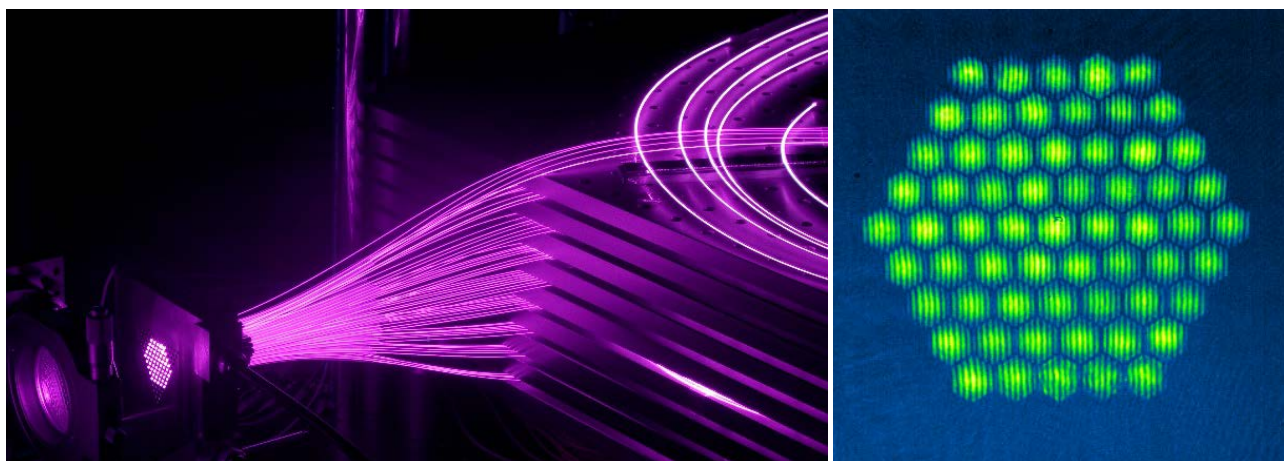
Figure 1. XCAN 61 Yb-doped fiber amplifier bundle (left) and near field interference pattern (right).
