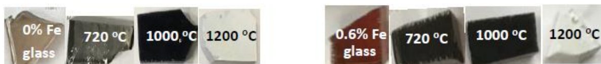
Figure 1. Photographs of undoped and 0.6 mol% \text{FeO} -doped initial glass and GCs obtained by heat-treatments at temperatures of 720 - 1200^\circ\text{C} indicated in photographs. The holding time is 6 h.
