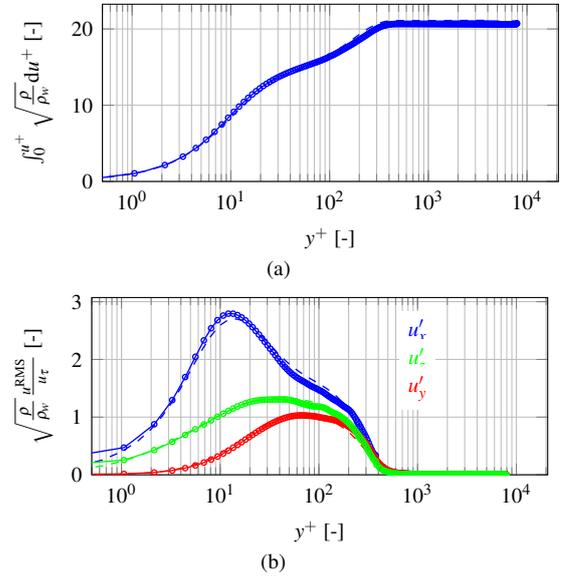
Figure 7: Time-averaged (a) and root-mean-squared (b) velocity at different longitudinal location. (—o—) Present LES. (---) DNS.
