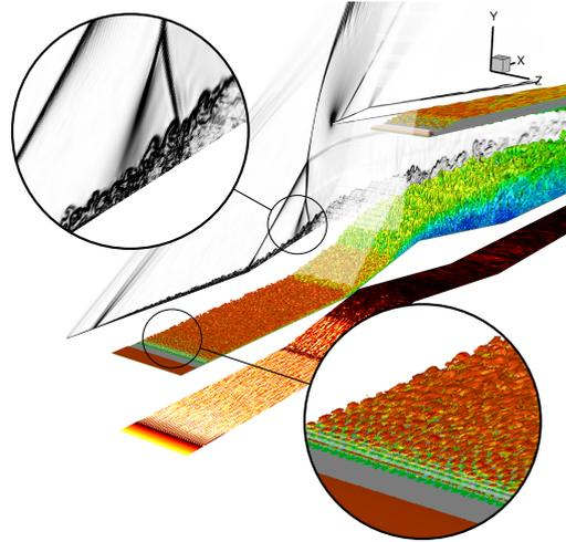
Figure 4: 3D view of the instantaneous flow field.  $Q$ -criterion colored by the axial velocity. (Left plane) Numerical Schlieren on a longitudinal slice cut. (Bottom surface) Wall skin friction coefficient.
