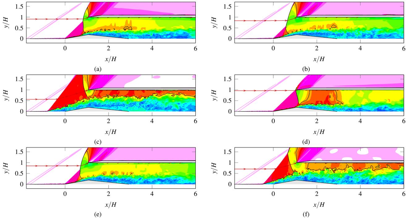
Figure 17: Instantaneous field of the Mach number at different characteristic times (see in Fig. 15c).
