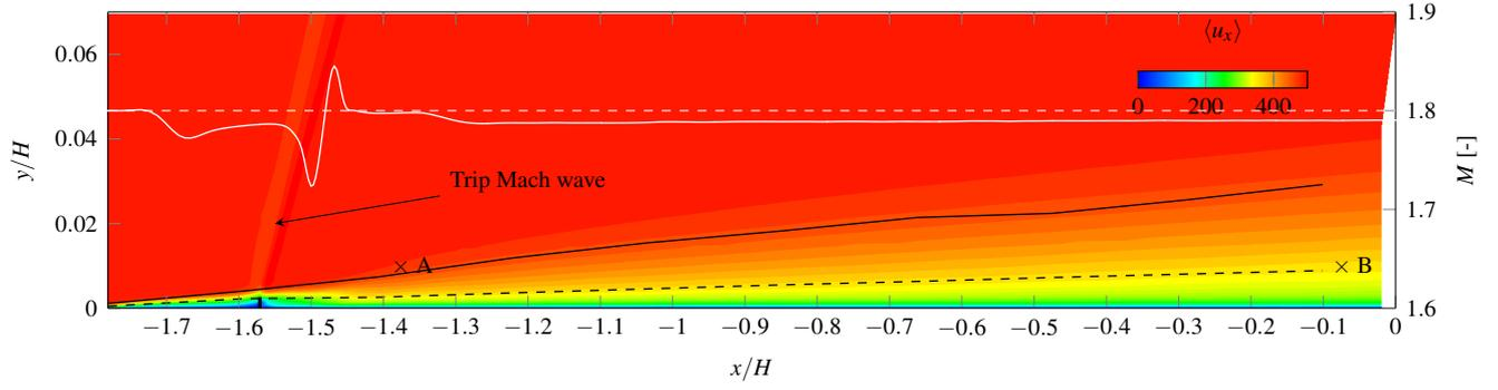
Figure 5: Close-up view on the upstream flat plate (vertical axis has been enlarged). Time-averaged longitudinal velocity field. (—) Boundary layer thickness  $\delta_{0.95}$ . (---) Boundary layer displacement thickness  $\delta_1$ . The vertical marker illustrates the trip location and real geometry. (Solid white line) Evolution of the Mach number at  $y/H = 0.065$ .
