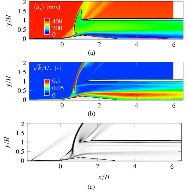
Figure 11: Mean (a) and fluctuating velocity (b) fields and (c) numerical Schlieren for  $TR = 0.72$ . (Black line) Sonic line. (Red line) Separation line ( $u_x = 0$ ).
