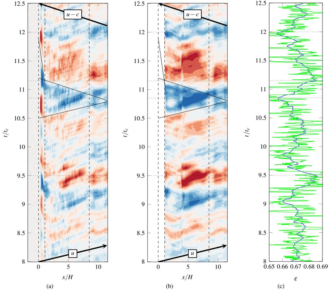
Figure 14: Filtered spatio-temporal map of the pressure fluctuation on the lower (a) and upper (b) walls at  $TR = 0.72$ . (c) Filtered (—) and unfiltered (—) time-evolution of the normalized mass flow ratio through AIP.
