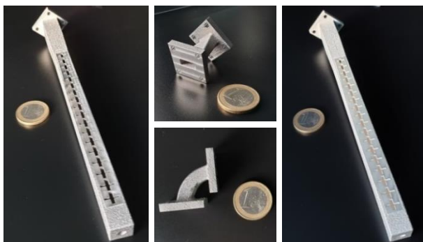
Fig. 6. Images of the prototypes (a) CP LWA before plating, (b) bend and twist for test (c) CP LWA after plating.
