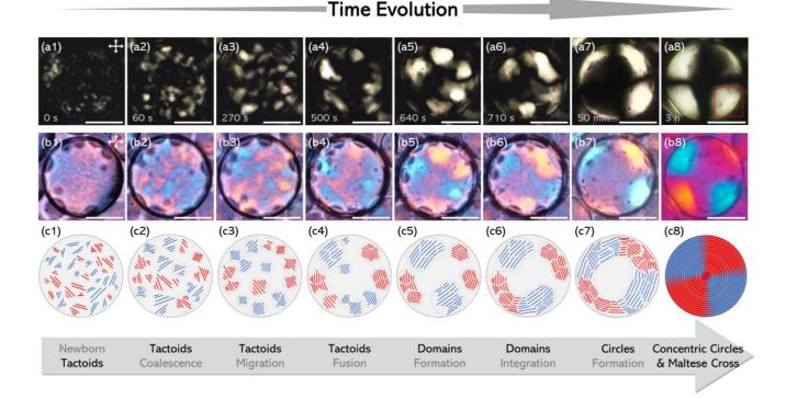
Figure 3. Typical POM images of time-series snapshots of TAA/CNC<sub>6%</sub> microdroplet without (a1-a8) and under lambda retardation plate (b1-b8) (scale bar = 50  $\mu$ m). Note that (a8) and (b8) was captured by using high magnification camera once equilibrium was reached. (c1-c8) Corresponding cartoon depiction of the microdroplet transforms from newborn tactoids to symmetrical concentric circles with Maltese cross structure.
