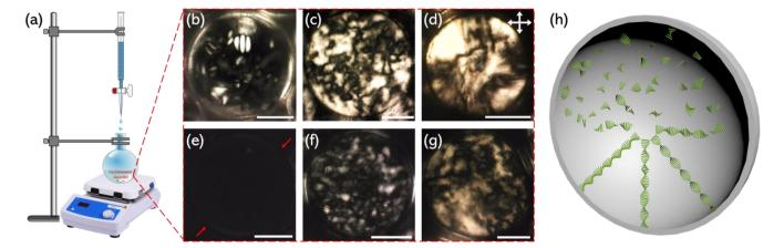
Figure 2. (a) Cartoon illustration of inverse microemulsion system. POM images of microdroplets of (b) CNC<sub>4%</sub>, (c) CNC<sub>6%</sub>, (d) CNC<sub>6%</sub>, (e) TAA/CNC<sub>4%</sub>, (f) TAA/CNC<sub>6%</sub> and (g) TAA/CNC<sub>6%</sub> (scale bars = 50 µm). (h) Schematic of microdroplet.
