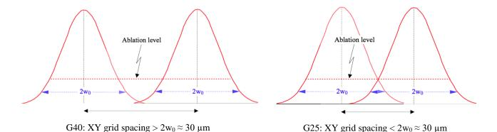
**Fig. 1.** G40 and G25 grid spacing of the Gaussian laser beam (waist  $2w_0$ ). According to the ablation level and the beam overlap, the surface should not be textured in the middle part with the G40 grid, unlike the G25 grid.
