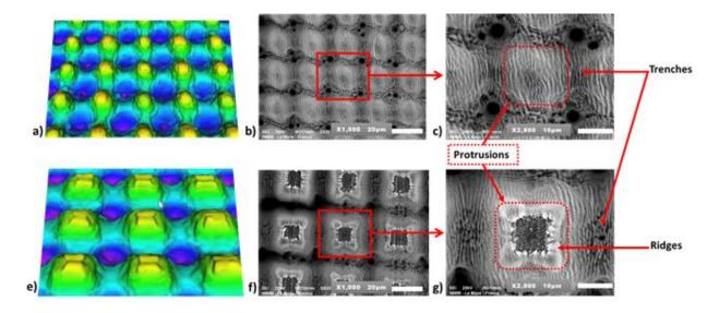
**Fig. 2.** Morphologic structure of femtosecond laser textured steel samples. The 3D profile of G25 substrate (a), with its corresponding SEM picture at x1000 (b) and x2500 magnification (c). The 3D profile of G40 substrate (e), with its corresponding SEM picture at x1000 (f) and x2500 magnification (g).
