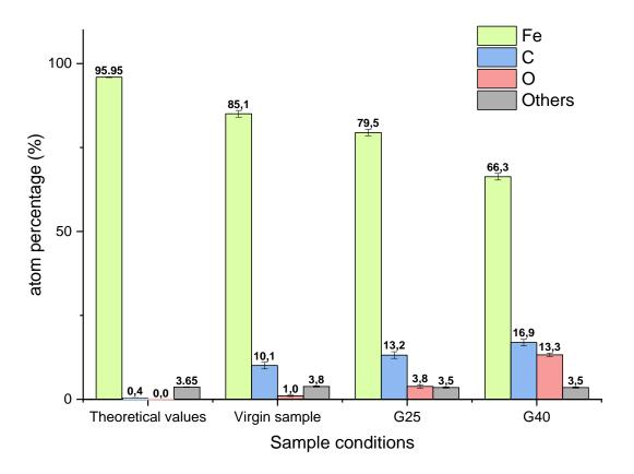
**Fig. 9.** Elemental percentage of iron, carbon and oxygen at the surface extracted from EDX mapping (Fig. 8) of the samples in different states compared to the datasheet values of 40CMD8+S. Virgin surface and two different laser patterning samples after 15 days of ageing.
