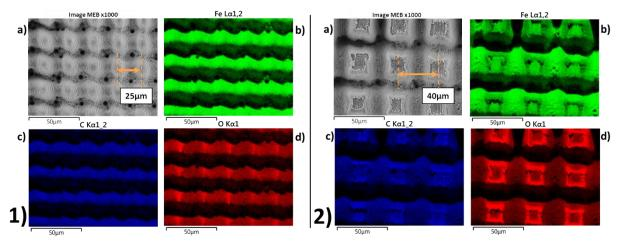
**Fig. 8.** SEM picture (a) and their corresponding EDX mapping (b to d) of the G25 (1) and G40 (2) patterns for each main element, 15 days after laser texturing.
