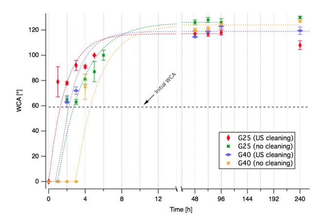
**Fig. 3.** Dependence on ageing time of the G25 and G40 wettability with or without ultrasonic cleaning. The dash line at 59° shows the initial WCA of a reference non-textured substrate.
