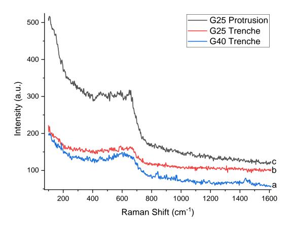
**Fig. 5.** Comparison of Raman spectra for the magnetite peak ( $Fe_3O_4 \ 662cm^{-1}$ ) in different locations of a textured substrate: (a) G40 trench, (b) G25 trench, (c) G25 protrusion.
