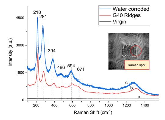
**Fig. 4.** Comparison of Raman spectra of 3 different steel surfaces: (a) Virgin sample, (b) ridge of a femtosecond laser textured protrusion a few hours after the laser treatment, (c) corroded sample in distilled water for 5 days.
