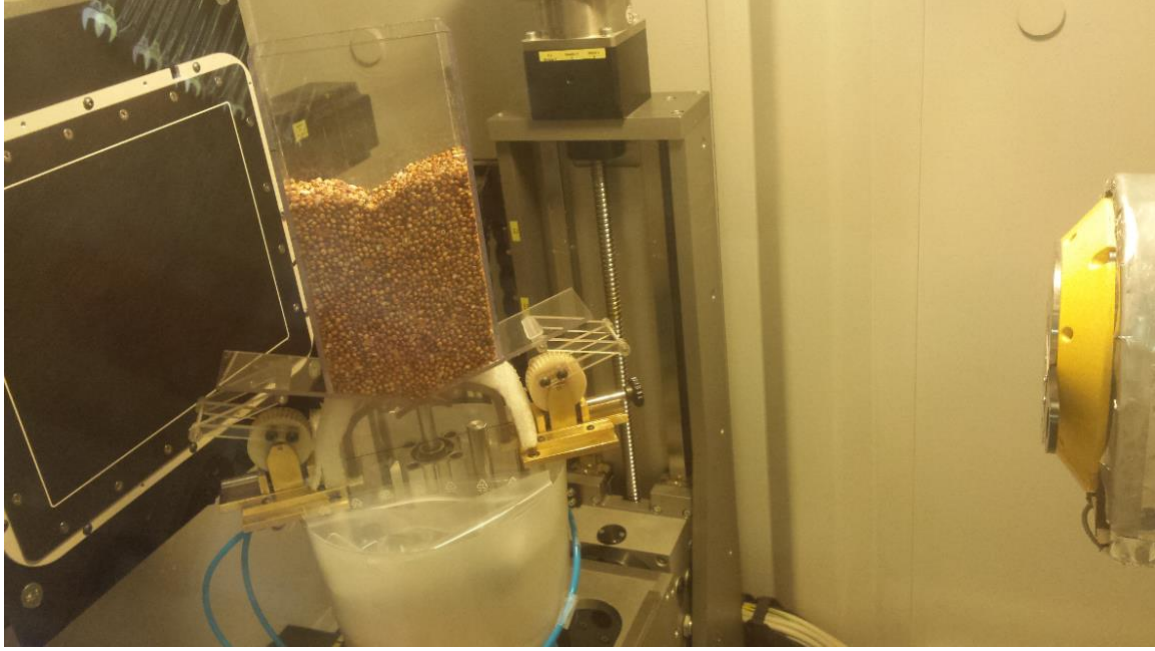
Figure 2. View of the interior of the X-ray tomography kit showing the silo configured for concentric funnel flow (material: sorghum).
