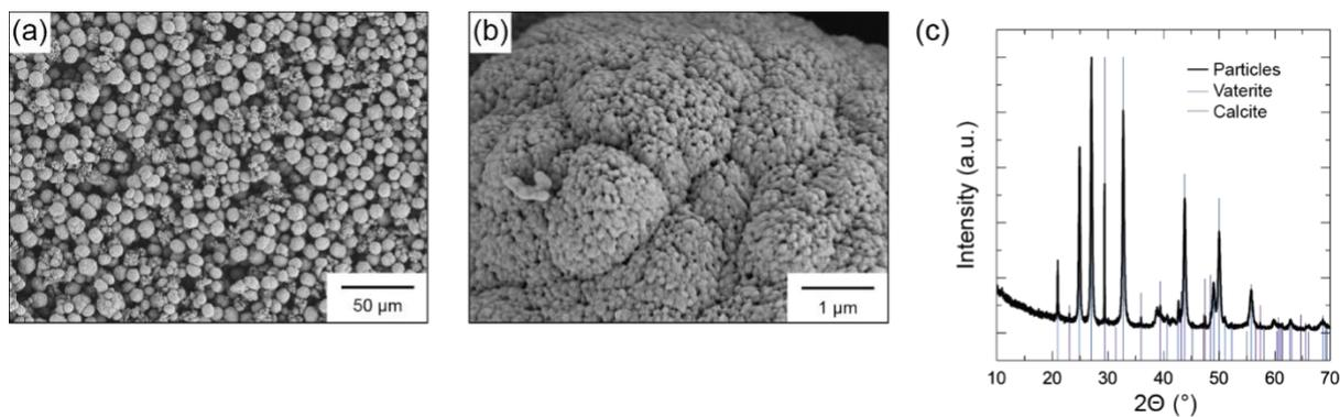
**Figure 2: Nanovaterite powder used for the preparation of compacts.** (a) Spherical vaterite agglomerates obtained after the precipitation reaction. (b) Hierarchical structure of the vaterite agglomerates, highlighting the presence of interconnected nanoparticles at smaller length scales. (c) X-Ray powder diffraction of the precipitated nanopowder, which indicates the predominant formation of vaterite crystals.
