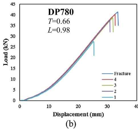
Fig. 11. Histories of load versus displacement strain for the (a) CP800 and (b) DP780 biaxial specimens interrupted at different strain levels.
