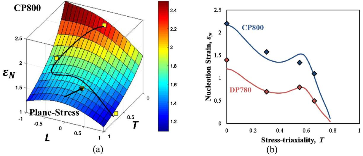
Fig. 24. (a) Representation of nucleation strain ( $\epsilon_N$ ) surface as a function stress triaxiality ( $T$ ) and Lode angle parameter ( $L$ ) for the CP800 steel. (b) The plane stress curve locus corresponding to the stress states and experimental data points are indicated by black line and square symbols, respectively.
