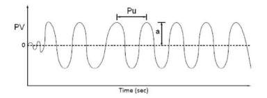
For a typical plant the oscillation obtained in the test occurring at the relay input is as shown in Figure 4. The critical frequency is taken as the measured frequency and the critical gain  $K_u$  is obtained by the formula,
