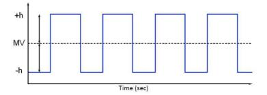
Figure 4. Output of closed loop control system with relay.
