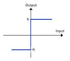
Figure 3. Relay output.
