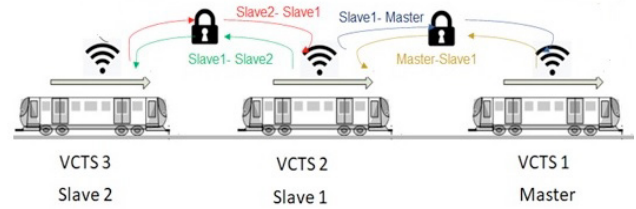
Fig. 4. Linear communication ( ((2 \times n-1) communication links)
