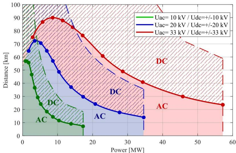
Fig. 4 – Break-even distance and power of point to point transmission in terms of losses for different voltage levels. Dashed area represents the power and distance range where DC transmission results in lower losses. The dashed line represents the limits of the transmission scheme (maximal current or maximal losses).
